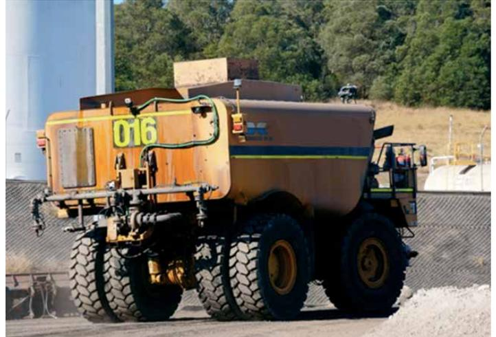
The key operating principle of the ADE Spray system is that it can spray a defined water application rate rather than an unknown 'high' or 'low' flow water output, thereby ensuring water output is controlled and greatly improving costs, manage water usage and efficiency.
