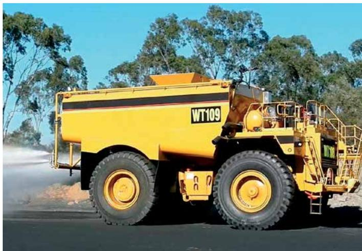
In 2013, ADE set out to solve the safety related issues of mine haul road watering with the development of the ADE Spray system. The purpose of the system is to suppress fugitive dust emissions, prevent truck slides and vehicle rollovers, and to deliver operational cost savings to mine operators through spraying haul roads more effectively and efficiently.
